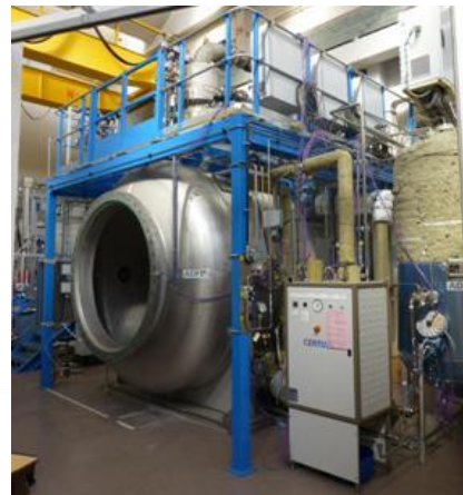
Illustration of PEARL facility designed to study debris bed reflooding
