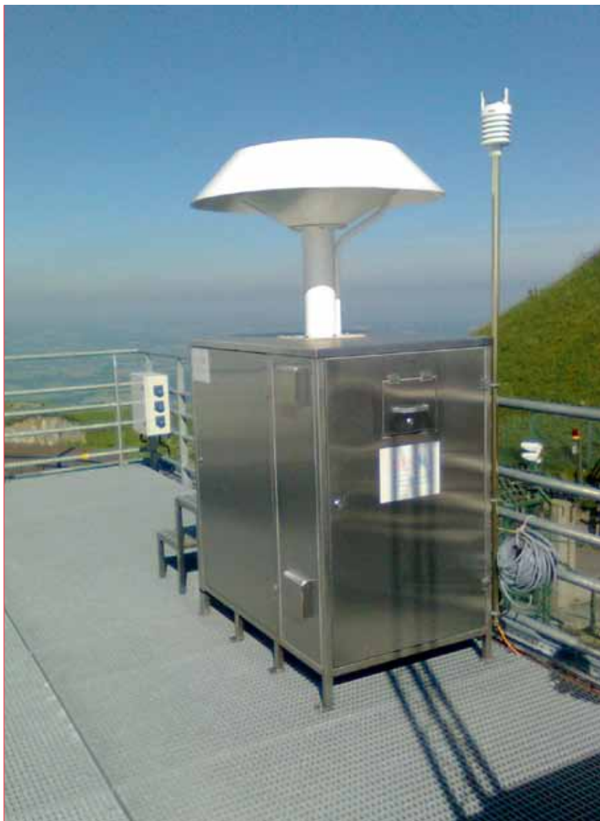
■ Figure III.24 - Very high-volume (700 m 3 /h) aerosol sampler in IRSN's OPERA-Air network (Puy-de-Dôme site in south-central France).
