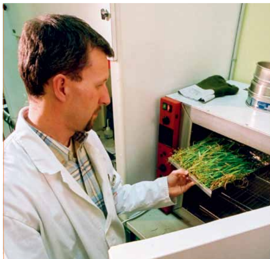
Figure V.144 - Oven drying of a grass sample
