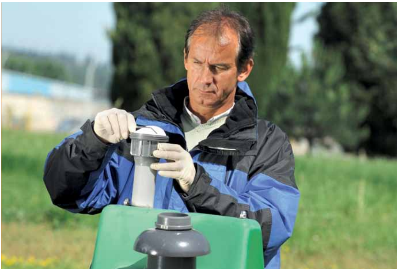
■ Figure V.30 - Recovery of the filter used for sampling atmospheric aerosols on the FBFC Romans-sur-Isère site
