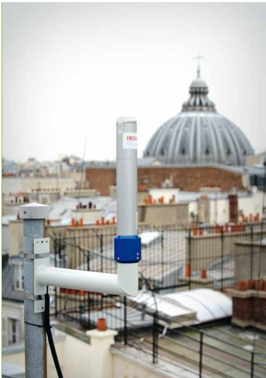
Figure 1.9 - New-generation IRSN Télérady monitor (for gamma radiation dose rate measurement) installed in Paris (French naval staff headquarters)
