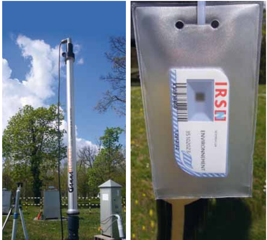
Figure IV.1 - Instruments used to measure the gamma dose equivalent rate in the atmosphere: on the left, an active device (Gamma Tracer probe from the EDF network) and on the right, a passive device (radiophotoluminescent (RPL) dosimeter).
