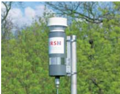
■ Figure X.6 - Probe for continuous monitoring of ambient gamma dose rate.
