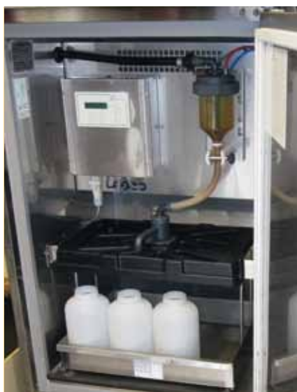
Figure IV.25 - Detailed view of an IRSN water sampler.
