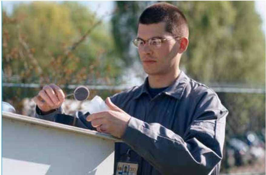
Figure VI.22 – Daily retrieval and conditioning of the aerosol filter.
