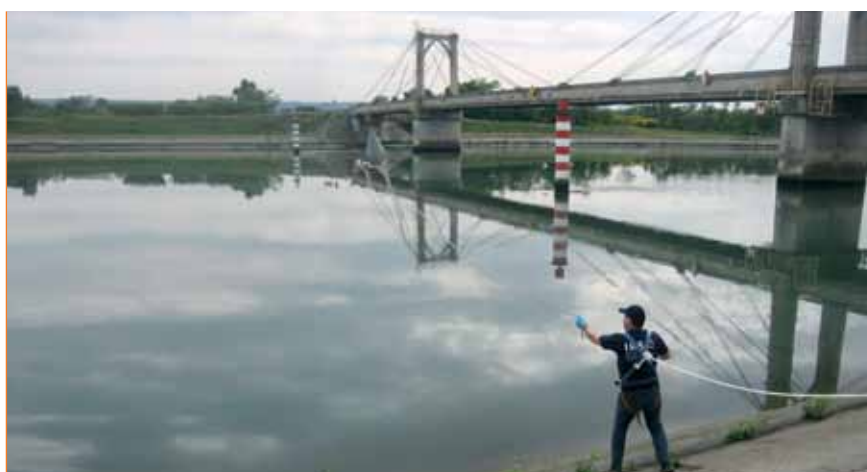
Figure V.26 - Sediment sampling in the Donzère-Mondragon canal upstream of the Tricastin nuclear site
