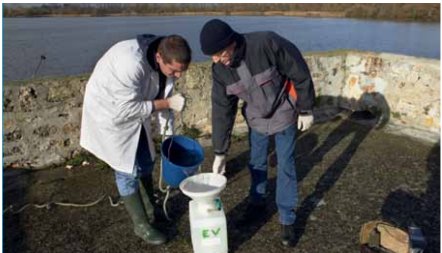
Figure VI.46 – Taking a water sample from the Étang Vieux pool near the Saclay site, for radiological and physicochemical analysis.
