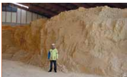
Figure VII.3 - Radium-bearing low-level long-lived waste stored at the Rhodia plant in La Rochelle.
