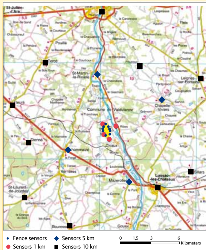
Figure IV.4 - Geographical distribution of ambient gamma dose measurement points around the Civaux nuclear power plant (EDF).
