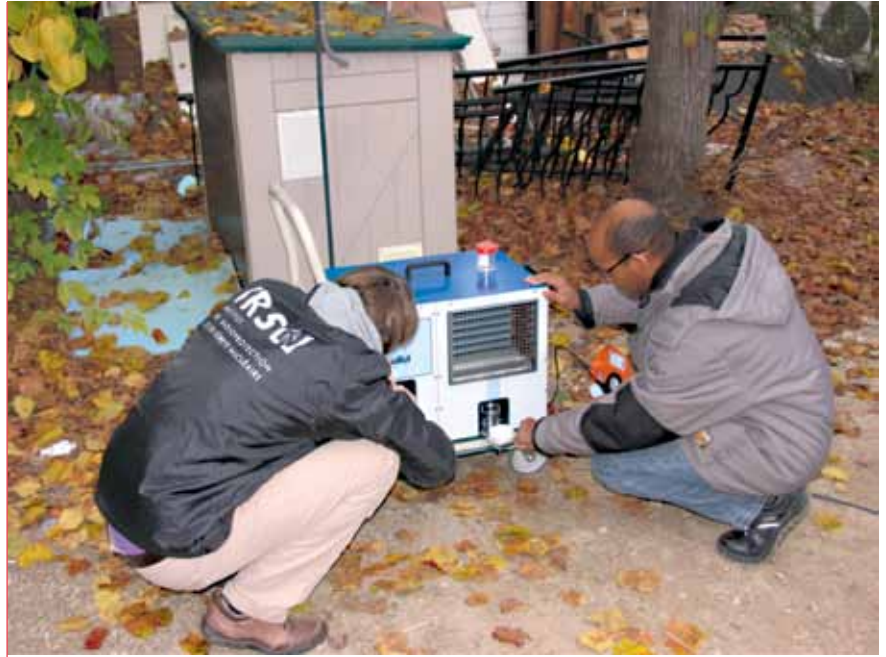
Figure III.17 - Sampling of water vapor in air with the H3R-7000 system in the courtyard of 2M Process.
