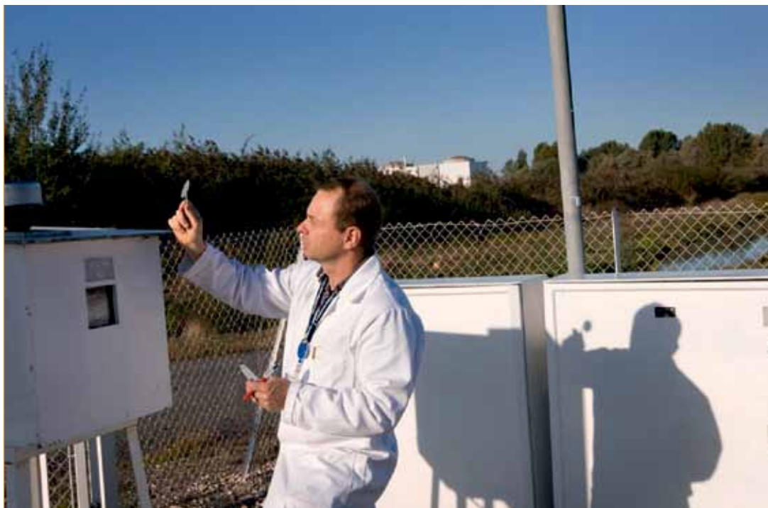
Figure V.70 - Recovery by an EDF technician of an atmospheric aerosol sample collected on a filter in the environment near the Le Blayais NPP
