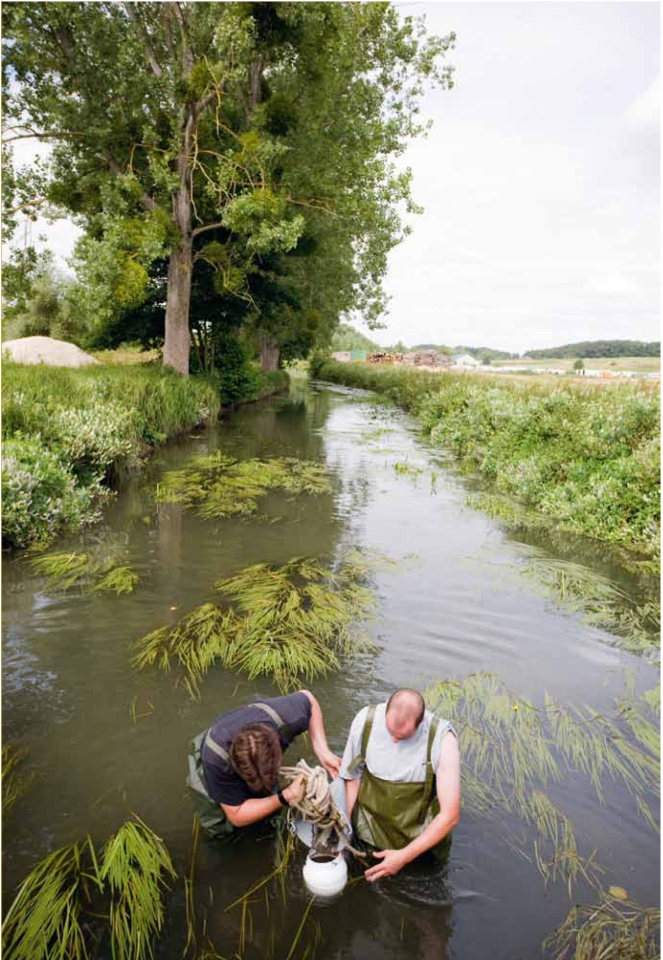
■ Figure IV.78 - Sampling sediments from a river using a Berthois cone.
