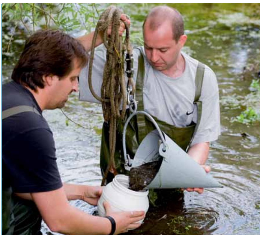
Figure VI.47 – Taking sediment samples in the Étang Vieux pool near the Saclay CEA center.
