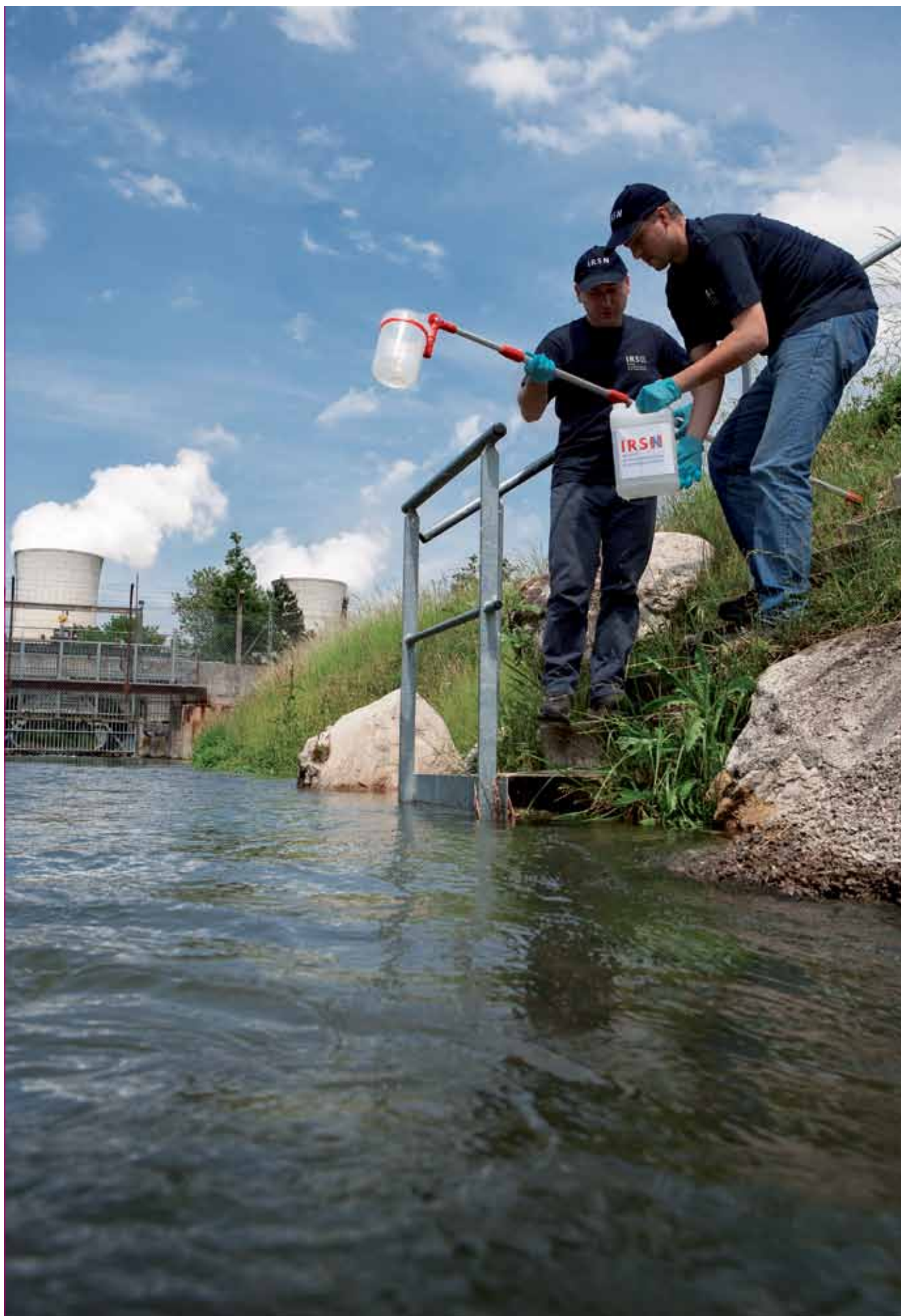
Figure VIII.10 - Using a telescopic boom to collect a water sample in the Gaffière river downstream from the Tricastin nuclear plant.
