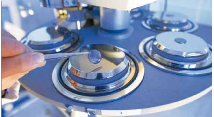
Figure I.14 - Spectrometry measurement on alpha spectrometry system with a grid ionization chamber
