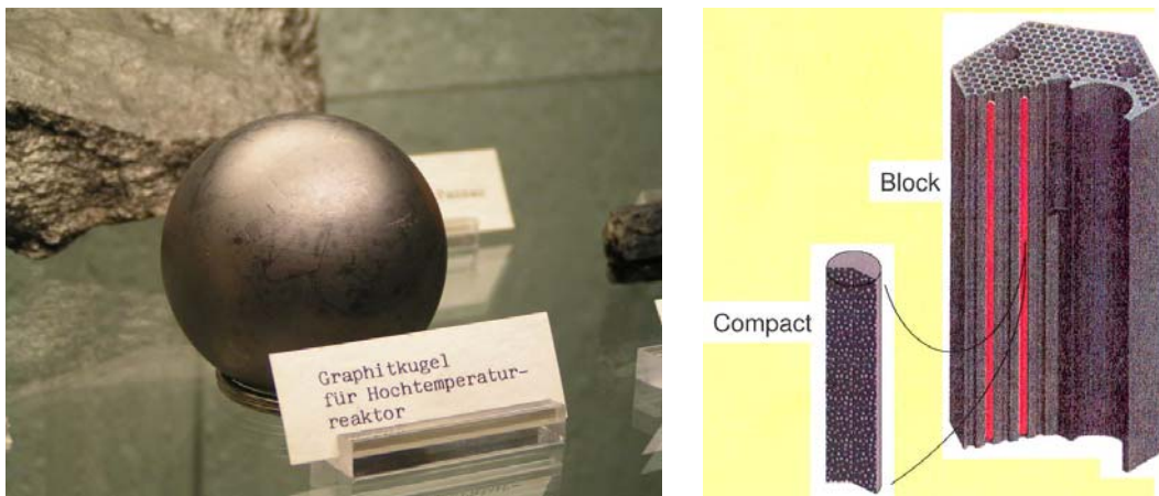
Figure 1: Left: a reactor pebble. Right: "compact" and fuel block for high temperature or very high temperature reactors.
