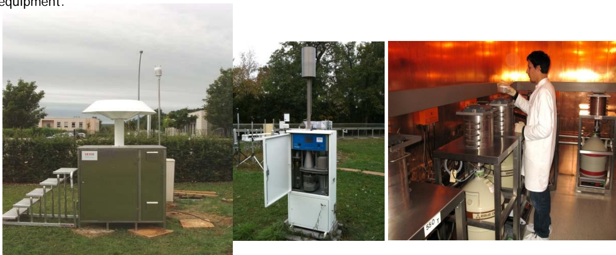
Figure 1 - IRSN OPERA-Air network equipment: very high flow rate aerosol collection station (TGD) on the right, intermediate flow rate aerosol collection station (Le Vésinet) in the centre, and shielded gamma spectroscopy room in the Orsay IRSN Laboratory.
