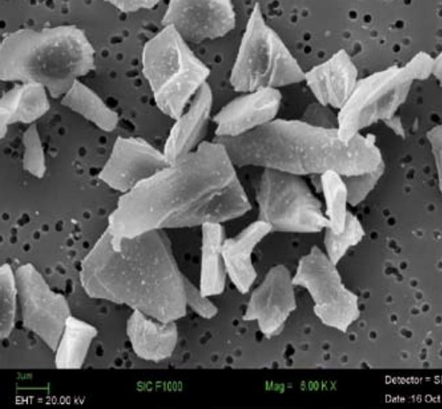
Carborundum micrography used in testing powder resuspension.
