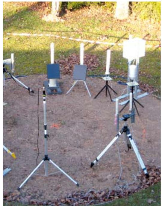
Platform used to assess ambient gamma dose rate measuring instruments selected to modernize the T el ery network.
