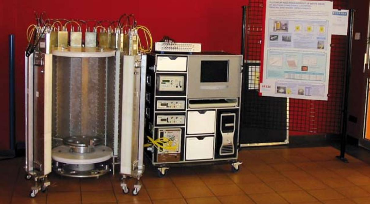
Equipment for measuring plutonium quantity in waste drums.
