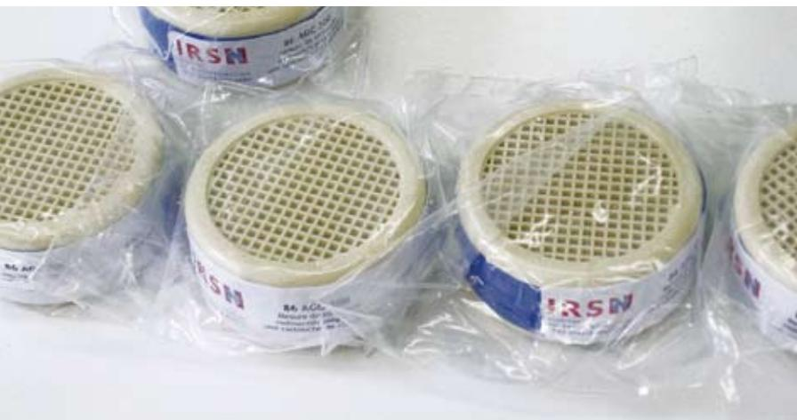
Filter cartridges with traces of radioactive iodine to be sent to laboratories participating in intercomparison test.
