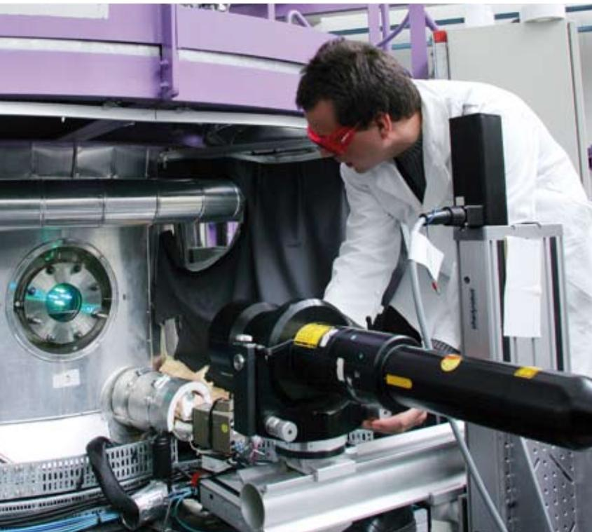
Laser velocimetry measurements in the TOSQAN facility.
