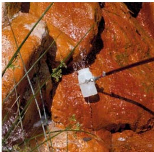
Sampling water downstream from a uranium mine.
