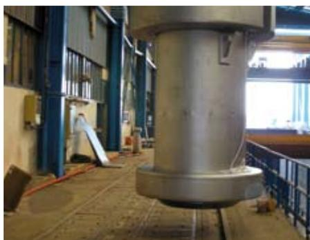
IR 800 irradiated fuel element transport package.
