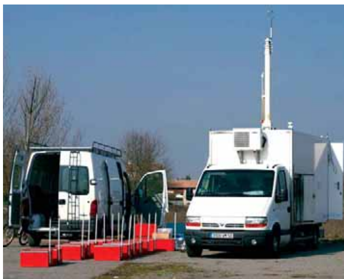
Micro weather station and SF 6 gas sampling devices used by the Octeville laboratory for the CAPITOUL project.
