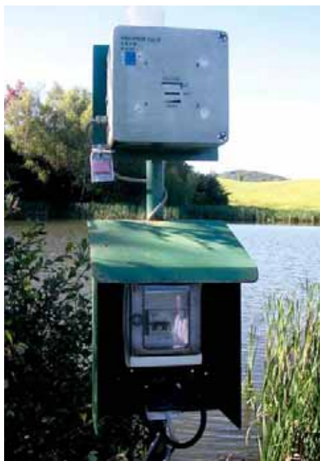
Dosimeter on the Cogema site to monitor the former mine site of Saint-Pierre du Cantal.
