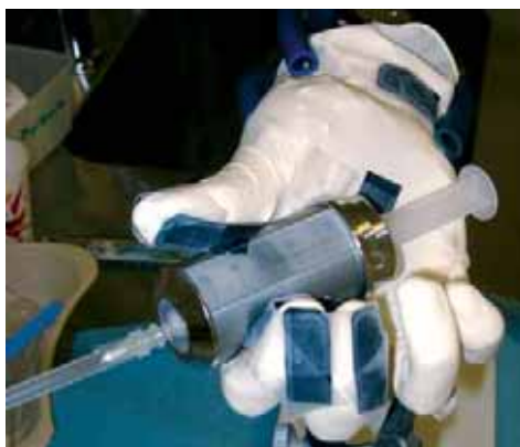
Installation of dosimeters to measure the exposure of fingers when using a syringe shield in nuclear medicine.
