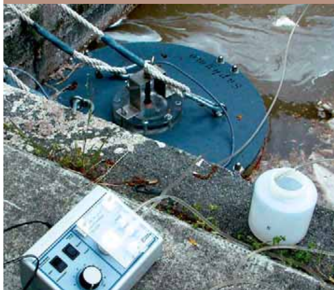
Portable Telehydro probe immersed at the exit of a waste water collector in a Toulouse hospital.
