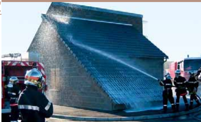
Testing of decontamination techniques on buildings by SDIS teams in the Cher department.
