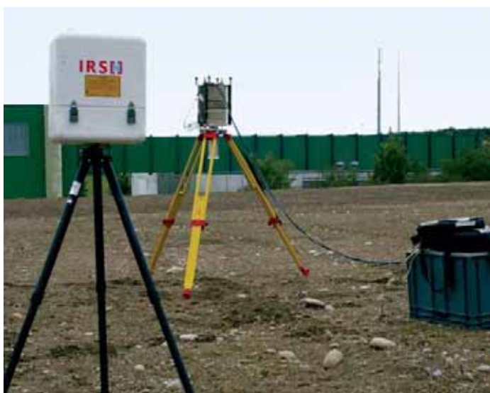
In situ gamma instrumentation near CERN to define the radioecological reference point (Geneva).
