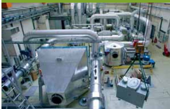
Full-scale blowing device to test the air flow and mechanical strength and compartmentation equipment behavior under pressure.
