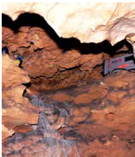
Devices to measure radon concentration in a cave.
