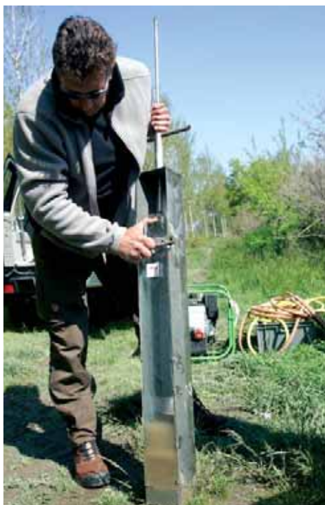
Sample core of sediment from the river Rhône (EXTREME project).
