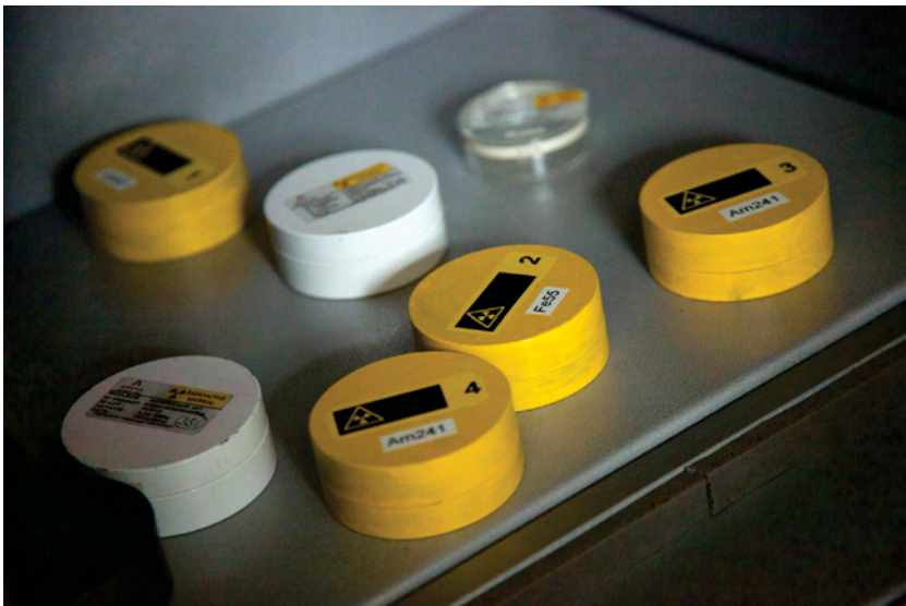
Figure 24. Sealed radioactive sources in their lead box, Université Toulouse III - Paul- Sabatier (France). © Albin Millot/IRSN.
