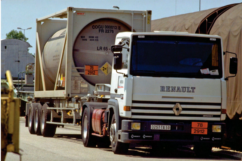
Figure 17. Truck transporting uranyl nitrate in an ISO standard LR 65 container. Manche. © EURODOC CENTRIMAGE, AREVA.
