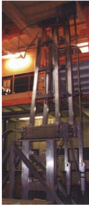
Figure 2.6. Telescopic device at the OSIRIS reactor used to carry out slow power ramps, according to IAEA Report 455. © DR.
