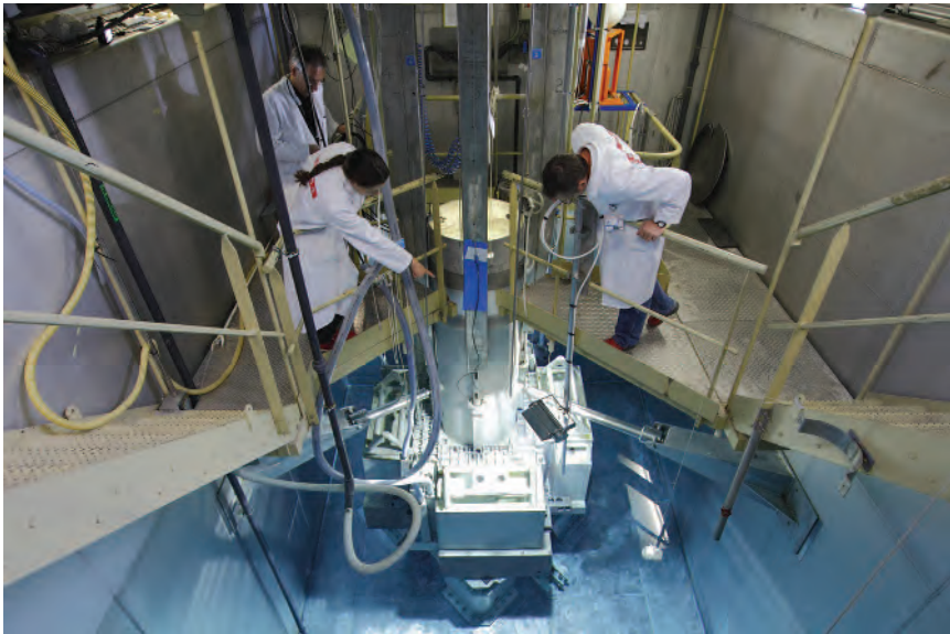
Figure 5.4. The MINERVE pool. Loading a sample into the central cavity to measure the reactivity effect using the “oscillation method”. © G. Lesénéchal/CEA.
