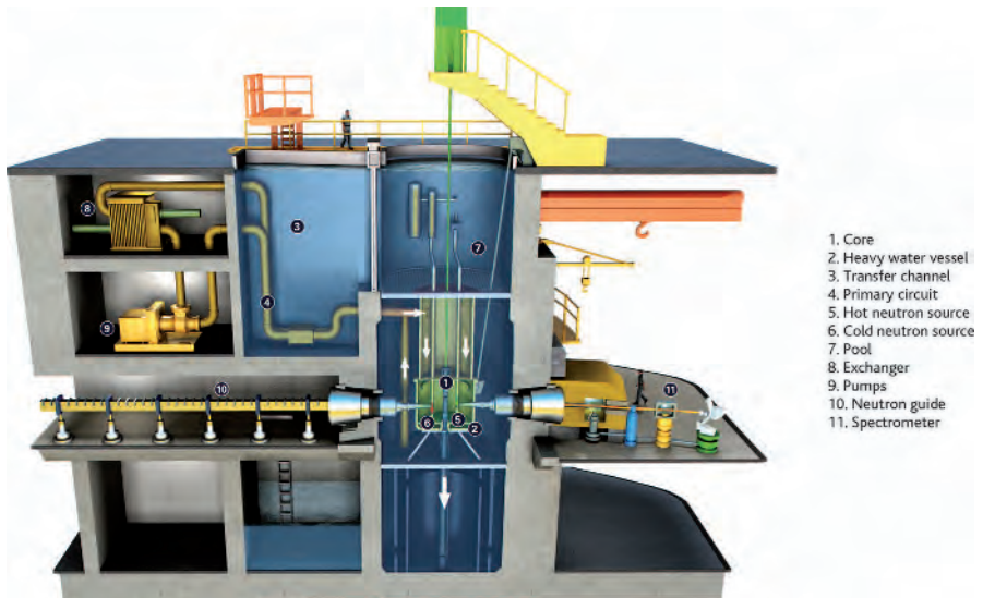
Figure 5.15. ORPHEE reactor: diagram of the reactor block, vertical section. © CEA.
