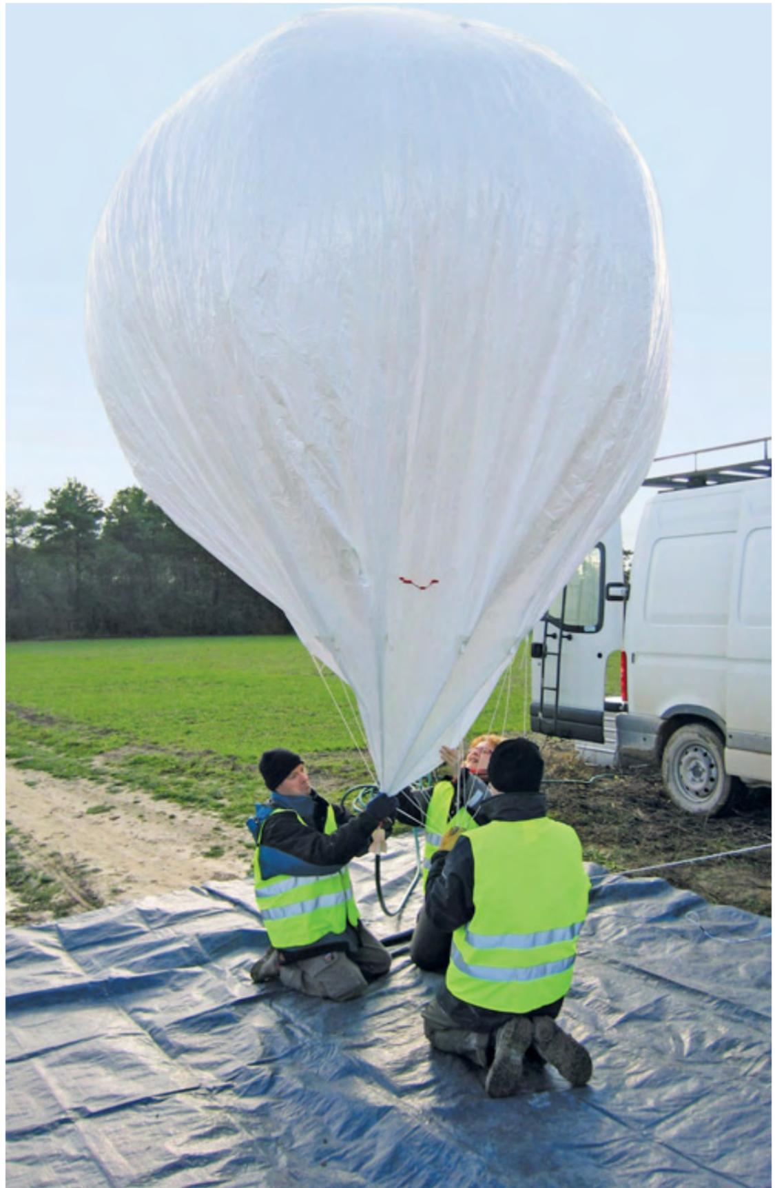
■ Preparing IRSN's captive balloon for high-altitude tracer gas measurements.
