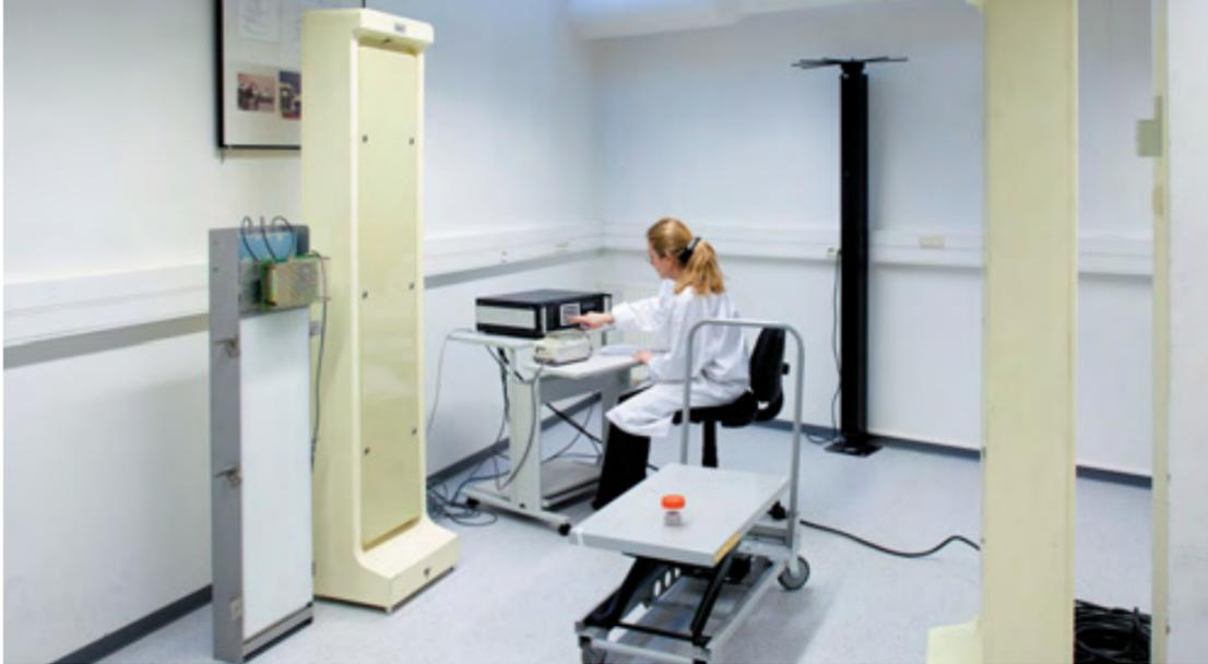
■ IRSN tests the performance of radioactive material detection barriers.
