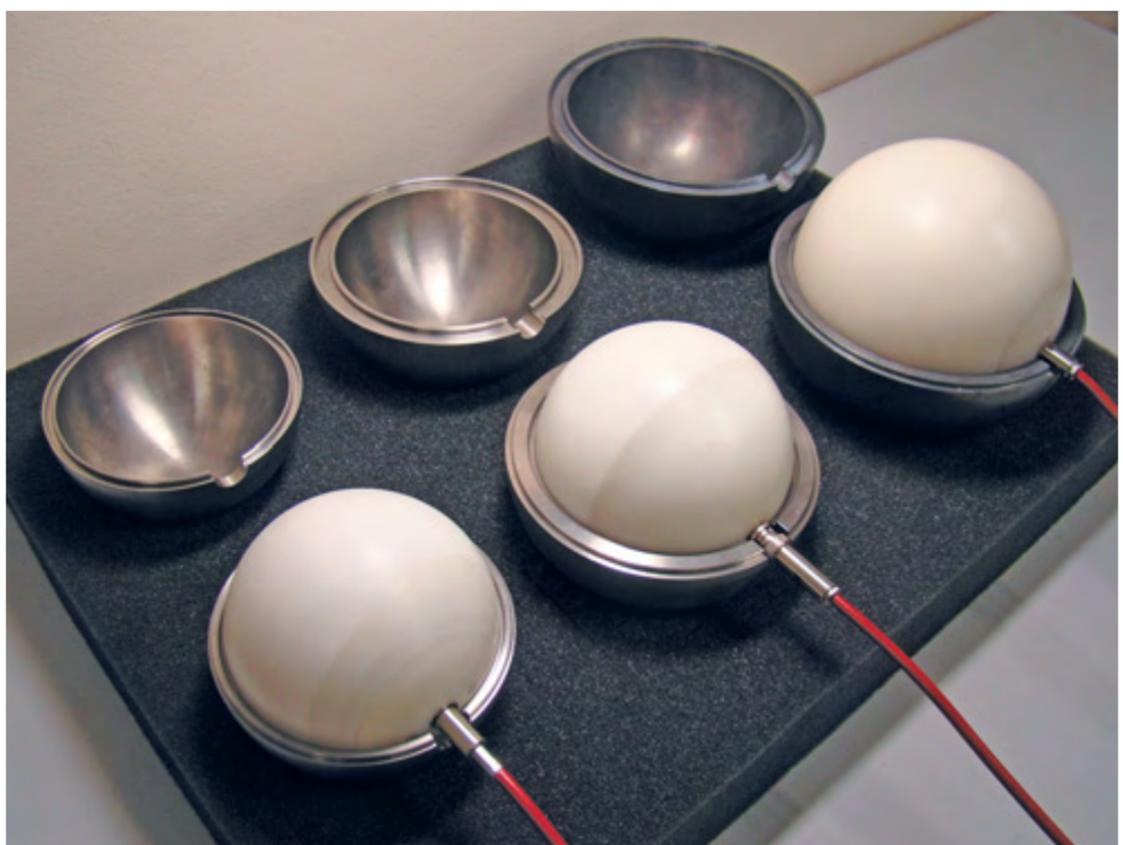
■ Bonner spheres with metal shells used in the spectrometer for measuring high-energy neutrons.
