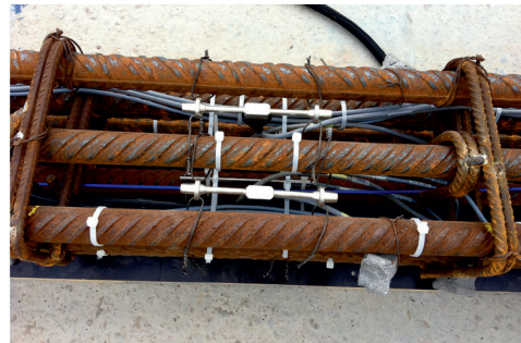
Figure 27.16. Left, diagram of a vibrating-wire extensometer. SFEN; right, view of two extensometers installed in a structural rebar grid before concrete is poured. EDF.
