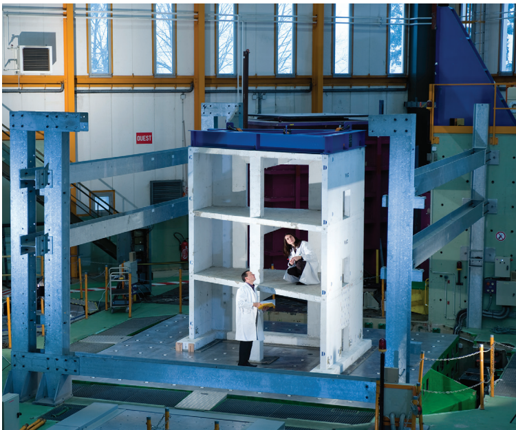
Figure 39.3. View of a nuclear building mock-up (such as an electrical building) for seismic simulation on CEA’s AZALÉE vibrating table. P. Stroppa/CEA.
